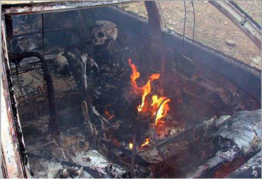
Photo 5: Fat absorbed by porous material burning in a limited area (Wick Principle). From: J. DeHaan and E. Pope, Combustion Properties of Human and Large Animal Remains 35
