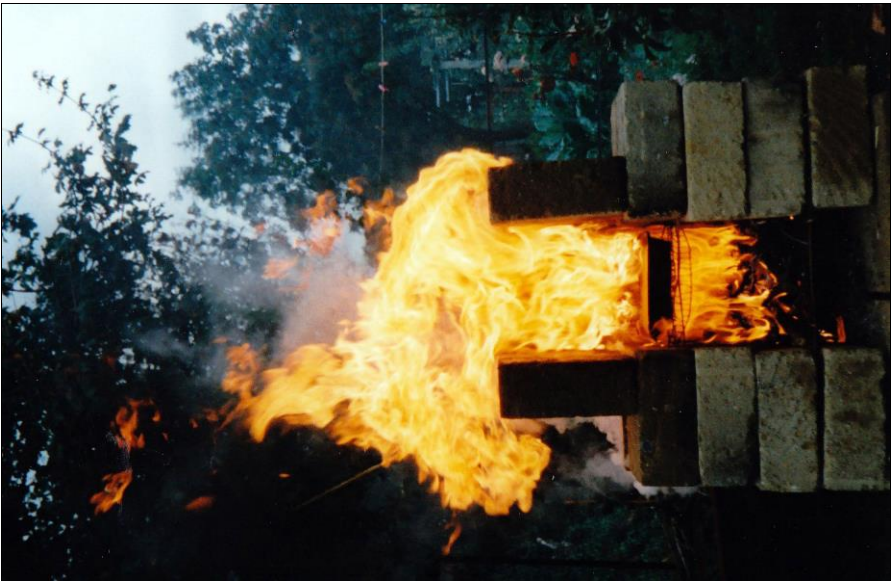
Photo 8 (sideways): Lard combustion experiment with pan above the combustion grid.
