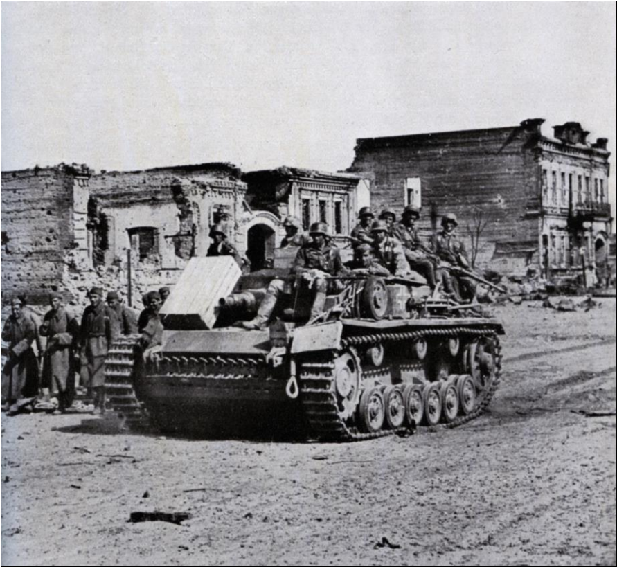
A self-propelled Sturmgeschütz III assault gun, consisting of a 75mm cannon mounted on the chassis of a Panzer III, passes Soviet prisoners in Stalingrad during the prolonged siege in late summer 1942. (Bundesarchiv)
