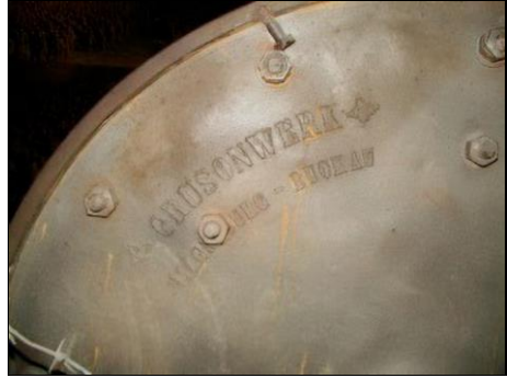
Fig. 8: Manufacturer's trademark on the drum of the ball mill. The star-shaped sign to the left and right of the word "Grusonwerk" was the trademark used by Gruson. Photograph: Private (2011)
