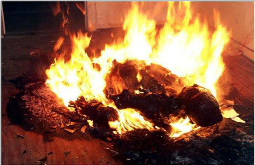
Photo 6: Fat burning completely and intensely when the temperature of the fire exceeds that of the inflowing fat. From: J. DeHaan and E. Pope, Combustion Properties of Human and Large Animal Remains 36
