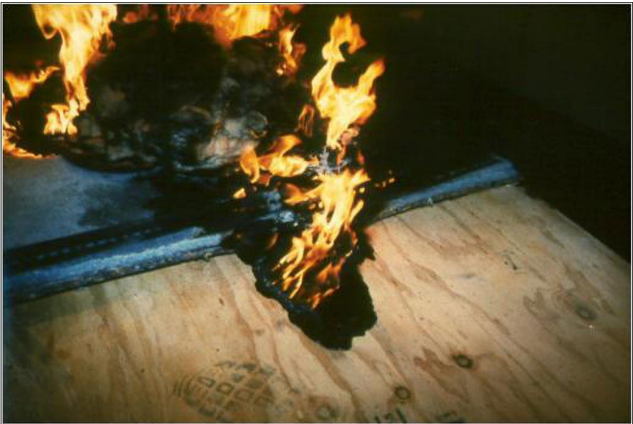
Photo 4: Fat burning at one single limited point within a pit of liquid fat (Wick Principle). From: J. DeHaan and E. Pope, Combustion Properties of Human and Large Animal Remains 34
